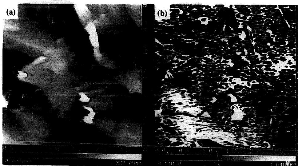
Fig. 5. 3 \mu\text{m} \times 3 \mu\text{m} simultaneous (a) contact AFM topography and (b) LM-FFM scans of KS-44/PVDF (90/10) anode sample. Darker areas in AFM scan correspond to lower areas. Darker areas in LM-FFM scan correspond to lower friction (KS-44) regions.
